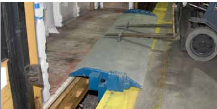
RAIL BOARD PLACEMENT
