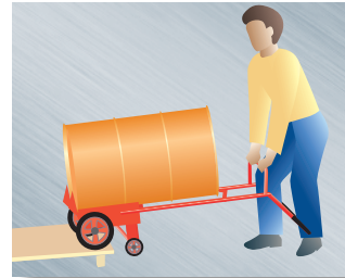
Use rear wheels to tip nose of Model 59 up onto pallet.
