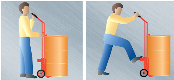
1. Lean truck against drum and drop hook over rim.
