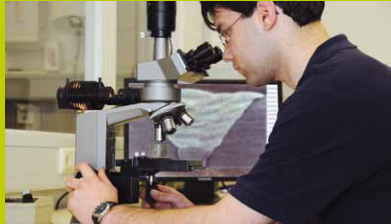
Microscopic weld seam inspection
