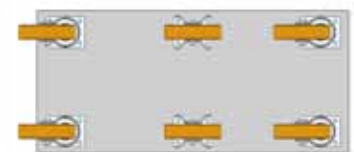
Four swivel and two fixed castors of identical mounting height
